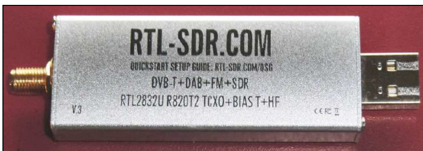
Fig 16: This is what the RTL-SDR.COM stick looks like. It is worth the small extra cost (see text)
