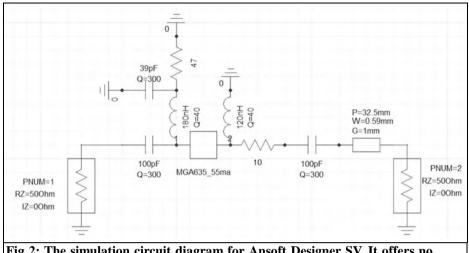
Fig 2: The simulation circuit diagram for Ansoft Designer SV. It offers no great mystery for the optimisation of noise figure and stability.
