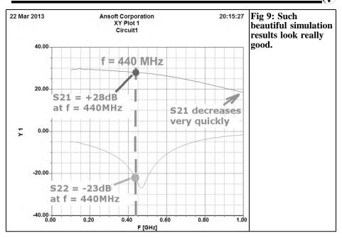
S21 will now decrease much faster with increasing frequency because of the inductance inserted in the output line since its reactance is also increasing. Therefore the stability factor "k" should be checked very closely up to 10GHz so that there are no unpleasant surprises, however Fig 10 is reassuring.
