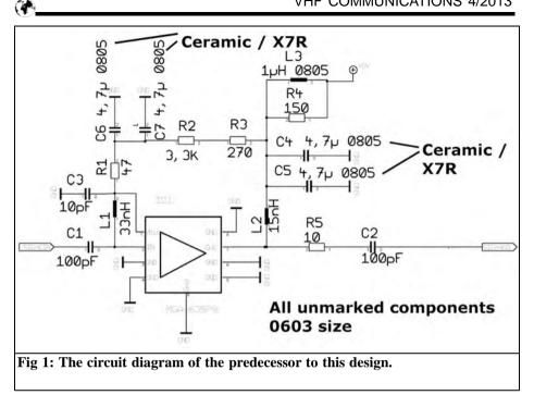
down in frequency has been examined for the possibilities of use on the 70cm band. This is more difficult, because the manufacturer of this MMIC only gives usage data above 1GHz therefore the MGA635-P8 documentation for the properties at low frequencies (e.g. noise parameters) is very, very poor. So, a request list was formulated and checked how far it can be met:
