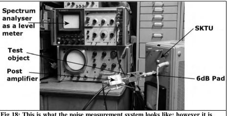
Fig 18: This is what the noise measurement system looks like: however it is important to understand the operation (see text).
