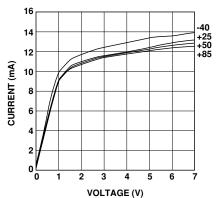
Figure 9. Device Current vs. Voltage.
