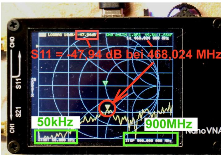
Now press the **Multi Function Switch (MFS)** to the right and hold it there. The marker moves from the start at 50kHz towards the higher frequencies. Try  $f = 468\text{MHz}$ , it will show 468.042MHz. The display has a scale on the left hand side with 10dB divisions as well as the top "Zero dB point".
