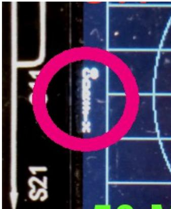
b) The currently active calibration will be shown in the middle of the left hand display border displayed as shown in the picture.
